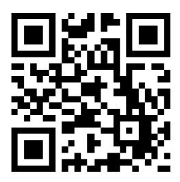
A 'quick response code' is a barcode that can be scanned by a smartphone with a camera which is then de-coded and converted to show the information behind it e.g. open a website or it could contain your boarding pass
