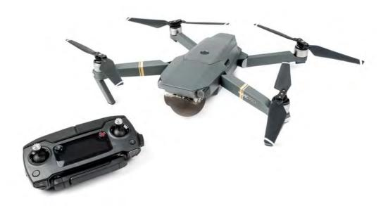
An unmanned aircraft that can be flown autonomously and beyond the line of sight.
